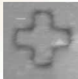
The smallest Swiss cross of the World is 25 nm wide and has been manufactured by etching trenches into a surface of a superconductor by STM (A. Takagi, PhD thesis, Geneva).
