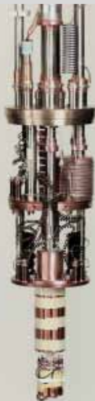
Low temperature part of a multipurpose cryostat insert for measurements below 1 K.
