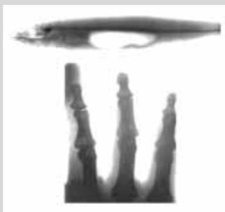
X-ray images of a fish and a human hand taken using Polaroid™ films placed behind the objects which were 30cm away from the nanotube x-ray source. Detailed bone structures are clearly resolved [1].
