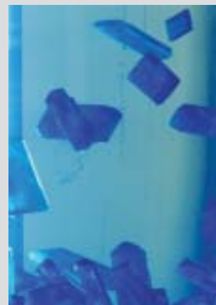
Micrograph of copper tartrate crystals grown by diffusion in sodium silica gel.
