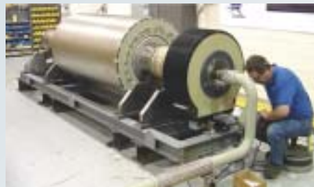
5MW Rotor Assembly with Exciter (Courtesy of American Superconductors)
