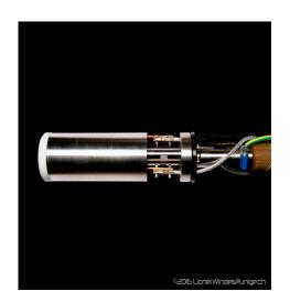
Details of the innovative superconducting coil, conceived and manufactured by researchers from UNIGE and Bruker BioSpin.
